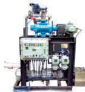
Dry Screw Vacuum Pump system for Solvent Distillation.
